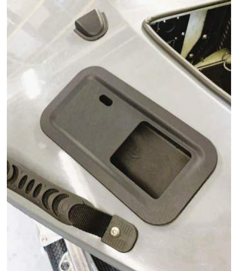
The plate cover installed on the Lightfish is 3D printed for durability and longevity to withstand the rigor of operating across the open ocean.
