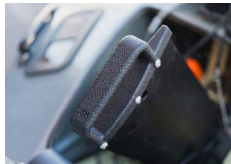
This functional handle installed on the Lightfish leverages additive manufacturing with digital textures to achieve efficiency and singularity in their designs.
