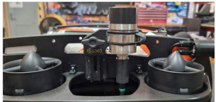
BlueROV-C with ISS360 Sonar lifted & ready for operation.
