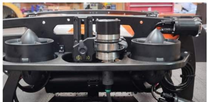
BlueROV-C with ISS360 Sonar stowed for transport.
