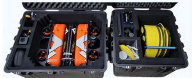
BlueROV-C with ISS360 Sonar stowed for transport.
